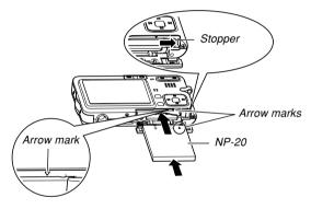
Push the bottom of the battery, and make sure that the stopper securely locks the battery in place.
